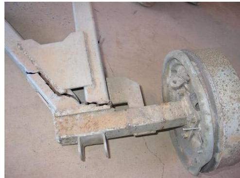
Apart from sustaining a broken caravan axle destroying the tyre in the process, all has gone well.
